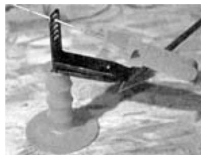
*Many sharpeners use hones attached to guides, such as the Gatco sharpener shown here, which allow the user to quickly put a razor edge on a broadhead.*
